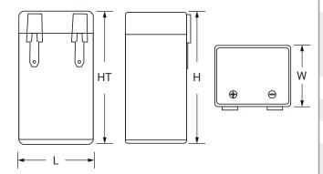
H: 2.99 (76) L: 1.69 (43) **W**: 1.46 (37) **HT**: 2.99 (76) Tolerances are +/- 0.04 in. (+/- 1mm) and +/- 0.08 in. (+/- 2mm) for height dimensions. All data subject to change without notice.
