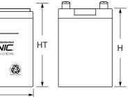
Tolerances are +/- 0.04 in. (+/- 1mm) and +/- 0.08 in. (+/- 2mm) for height dimensions.
