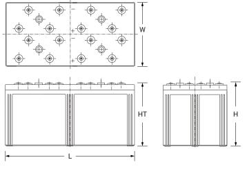
**L:** 27.90 (709) **W:** 13.80 (350) **H:** 13.62 (346) **HT:** 13.66 (347) Tolerances are +/-0.04 in. (+/-1mm) and +/-0.08 in. (+/-2mm) for height dimensions. All data subject to change without notice.
