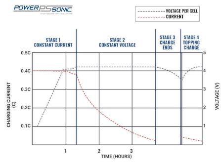
Stage 1 battery charging is typically done at 30%-100% (0.3C to 1.0C) current of the capacity rating of the battery. Stage 1 of the SLA chart above takes four hours to complete. The Stage 1 of a lithium battery can take as little as one hour to complete, making a lithium battery available for use four times faster than SLA.
