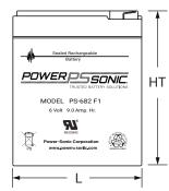
L: 3.86 (98) W: 2.20 (56) H: 4.65 (118) HT: 4.72 (120) Tolerances are +/- 0.04 in. (+/- 1mm) and +/- 0.08 in. (+/- 2mm) for height dimensions. All data subject to change without notice.
