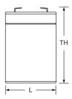
2.76 (70) W: 1.86 (47) 3.94 (100) TH: 4.17 (106) Tolerances are +/- 0.04 in. (+/- 1mm) and +/- 0.08 in. (+/- 2mm) for height dimensions. All data subject to change without notice
