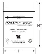
11 4.25 (108) 2.80 (71) 5.55 (141) W: H: HT: 5.55 (141) Tolerances are +/- 0.04 in. (+/- 1mm) and +/- 0.08 in. (+/- 2mm) for height dimensions. All data subject to change without notice.
