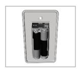
3. Make necessary DIP switch adjustments.
