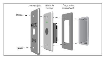
5. Secure with the provided screws (#6-32 flathead) and test functionality.
