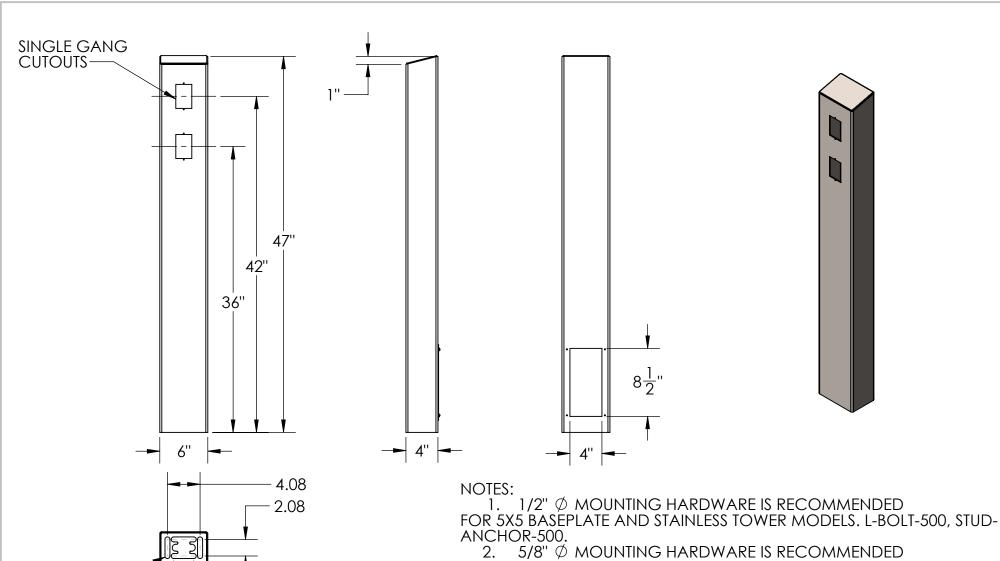
FOR 8X8 BASEPLATE, 12X12 BASEPLATE, AND BOLLARD STYLE **BASEPLATE**
