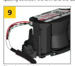
Plug the main harness into sensor at closest port.
