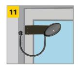
Mount the sensor to the arm. Plug the secondary sensor harness into the sensor. Route Primary Harness, and then install Door Loop and Cap onto the jamb.
