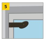
Secure the mounting arm with screws provided in the LZR-microscan kit. Cover the screws with the provided caps. Install the nylon spacer (Allen head end at the front of the arm), and adjust to fit for spacing between the arm and the door.<sup>2</sup>
