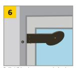
Drill 1/2" wire passage holes into jamb where Door Loops will be installed.
