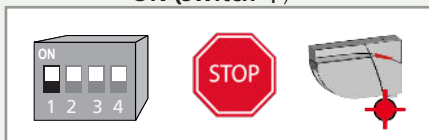
RELAY 1: STOP-impulse on swing side of door
