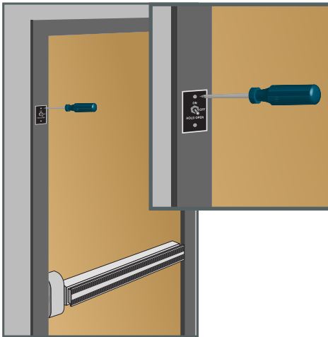
ON / OFF / HOLD OPEN Switch installed
