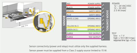
Sensor is intended to be monitored for proper operation by the door operator or system.
