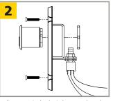
Adjust switch height on bracket until the cam triggers positively when rotated.
