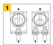
Select cam shape for keyswitches. *Mortise cylinder and second switch sold separately.*
