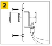
Adjust switch height on bracket until the cam triggers positively when rotated
