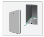
4. If <u>retrofitting</u>, cut off existing connectors (e.g. flag connectors) and strip the wires. If <u>new installation</u>, simply strip the wires.
