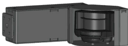
Finished assembly with LZR sensor installed
