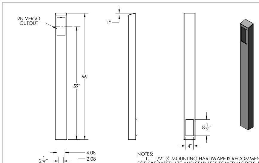
1. 1/2" ∅ MOUNTING HARDWARE IS RECOMMENDED FOR 5X5 BASEPLATE AND STAINLESS TOWER MODELS. L-BOLT-500, STUD-ANCHOR-500.
