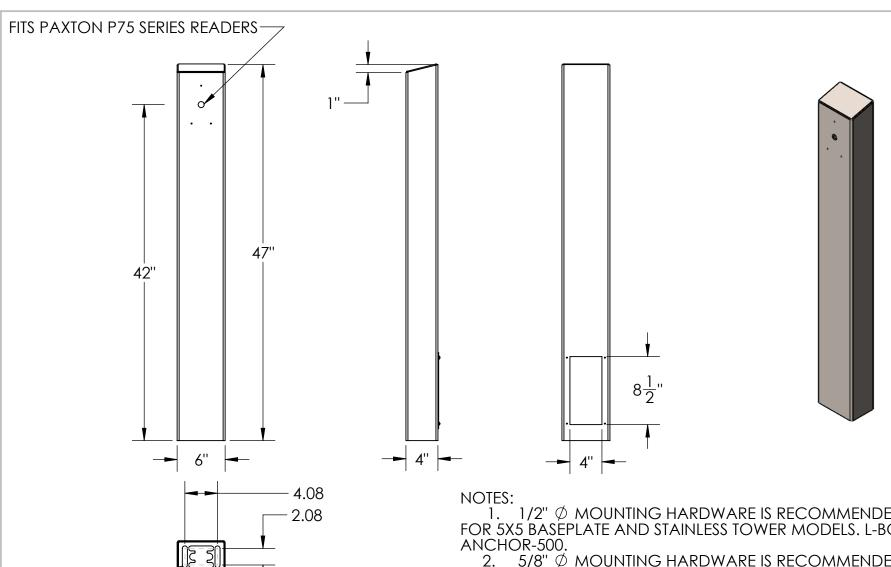
1. 1/2" Ø MOUNTING HARDWARE IS RECOMMENDED FOR 5X5 BASEPLATE AND STAINLESS TOWER MODELS. L-BOLT-500, STUD-
