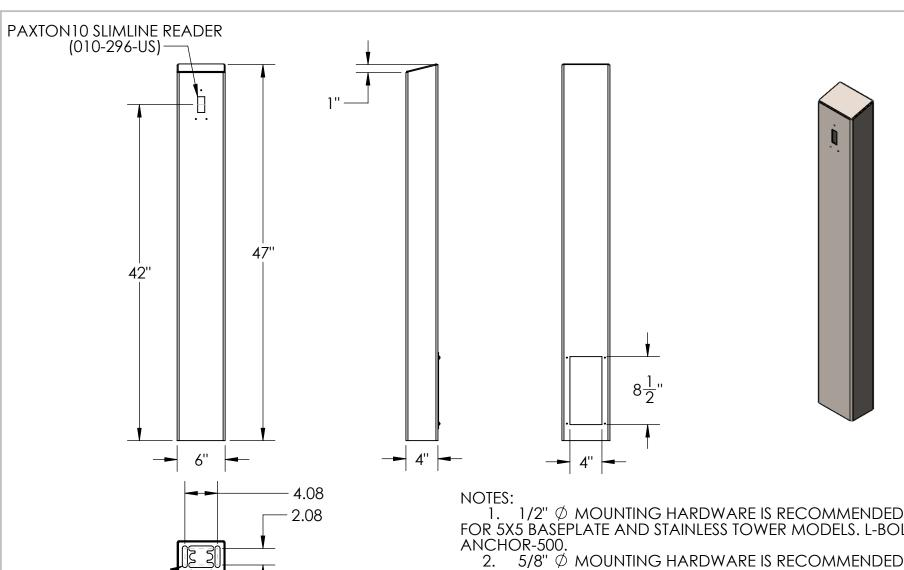
FOR 5X5 BASEPLATE AND STAINLESS TOWER MODELS. L-BOLT-500, STUD-
