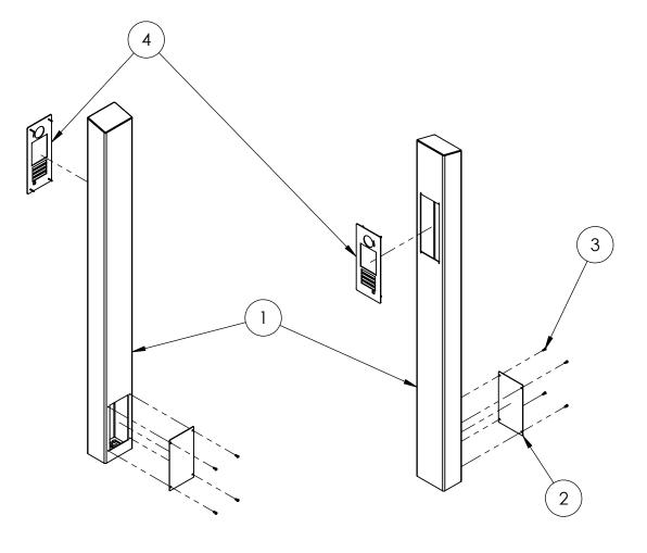
NOTES: 1. FACE PLATE BY AIPHONE MOUNTS TO THE FRONT OF THE TOWER WITH THREADED STUDS.
