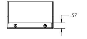
NOTES: 1. MATERIAL OF CONSTRUCTION IS MILD STEEL COATED IN 2-4 MILS BLACK WRINKLE POWDER COATING. 2. CUTOUT FOR HID 6005 PROXPOINT PLUS READER.
