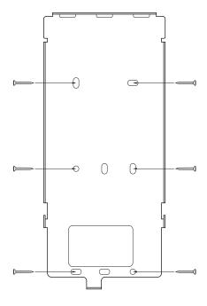
• If installing FaceStation F2 on a concrete wall, drill holes, insert PVC anchors, and fix them with fixing screws.
