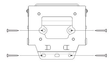
• If installing FaceStation 2 on a concrete wall, drill holes, insert PVC anchors, and fix them with fixing screws.
