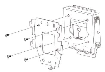
**4** Install FaceStation 2 onto the fixed bracket.
