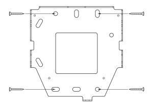
• If installing FaceStation 2 on a concrete wall, drill holes, insert PVC anchors, and fix them with fixing screws.
