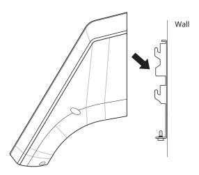
**4** Connect FaceStation 2 to the bracket by rotating the product fixing screw of FaceStation 2.
