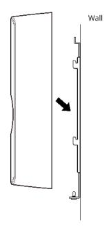
**3** Connect BioEntry R2 to the bracket by rotating the product fixing screw.
